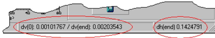
With a symmetrical cam profile, it is sufficient to achieve a velocity value of zero at the zero-degree point, since by the nature of the symmetric cam the velocity at the closing ramp will now match as will the lift.
